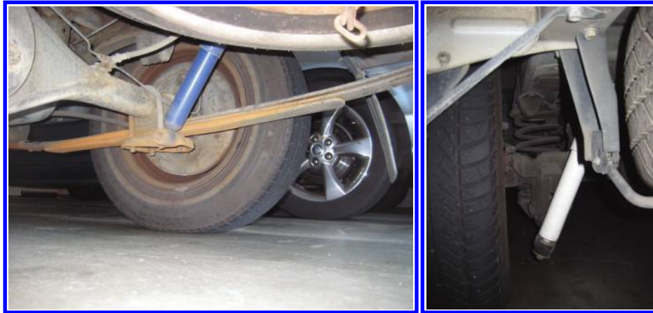
Figure 2.3: Typical spring-damper assembly of automobile suspension systems.
