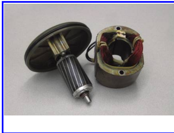
Figure 6.9: An AC induction motor's stator and rotor. The rotor is a simple non-magnetic cage with no power supplied to it. AC power is supplied to the stator coil only.
