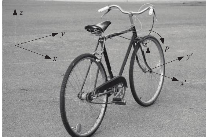
Figure 3.10: A moving frame and its motion relative to a fixed frame.
