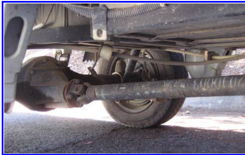
Figure 5.16: The polar moment of the area increases significantly as the shaft is made hollow but with the same area.
