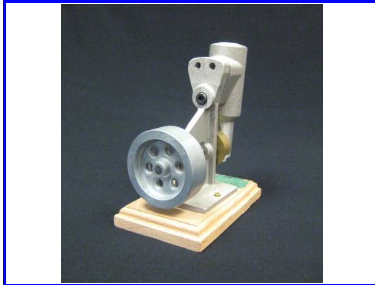
Figure 5.24: A typical flywheel is designed to have a larger mass moment of inertia without being too heavy by pushing most of the material outwardly to the rim.
