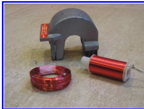
Figure 6.2: A permanent magnet and coils (when electricity flows through them) create a magnetic field around themselves.
