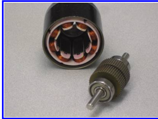
Figure 6.21: A hybrid stepper motor and its rotor and stator construction.
