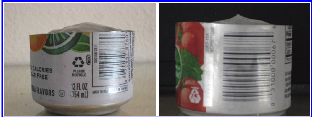
Figure 1.2: In a metal container, as water freezes around the perimeter towards the center, it expands and pushes the water level up slowly, creating a conical shape with an apex.
