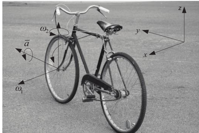
Figure 3.26: Rotations of a bicycle's tires and handle-bar and the resulting acceleration.
