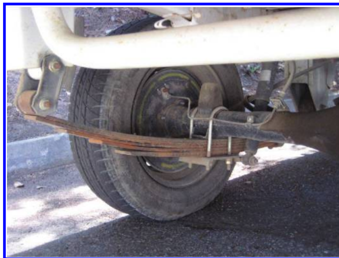
Figure 5.4: A leaf spring used in a truck.
