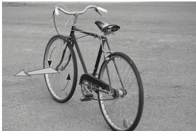
Figure 3.7: A bicycle's tire rotations can be specified by a vector.
