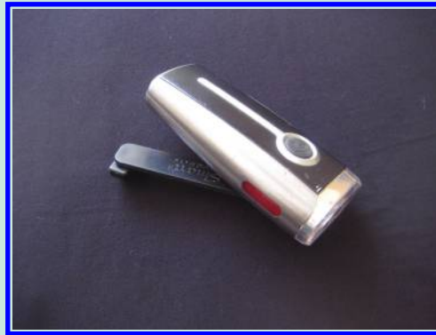
Figure 1.5: In this flashlight, a crank is used to rotate a generator in order to convert mechanical energy into electrical energy. This is either stored in a rechargeable battery or in a large capacitor.
