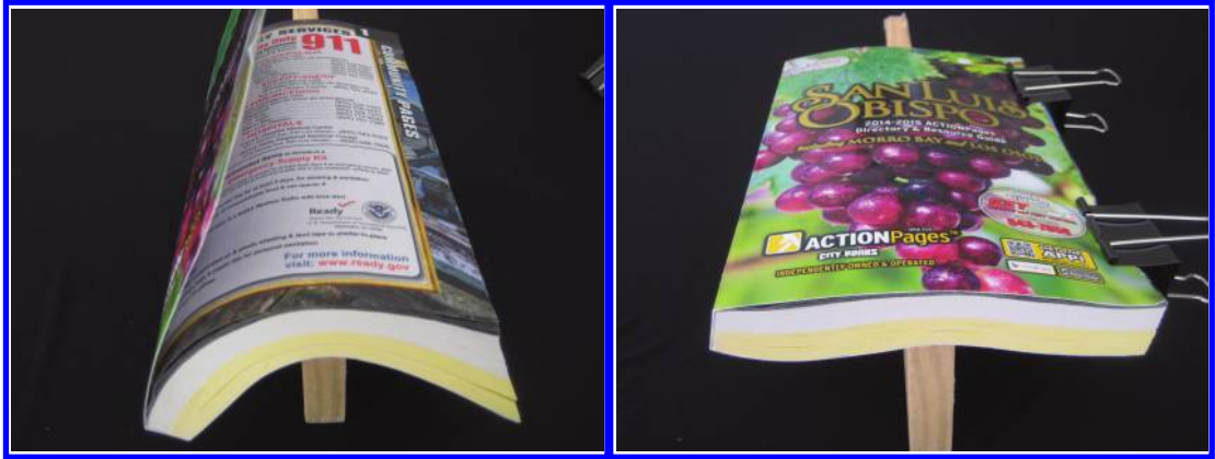
Figure 5.5: When the pages of a telephone book are prevented from sliding over each other, it does not bend as much due to the differences in second moments of the area.
