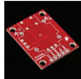
(b) Sparkfun joystick (COM-09032) and breakout board (BOB-09110)
