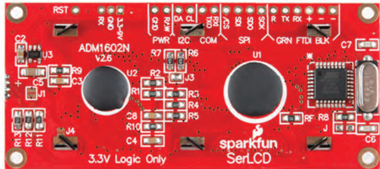
Figure 10.10: MSP430FR2433 interface to Sparkfun’s LCD-14072 display. (Illustration used with permission of Sparkfun Electronics ( www.sparkfun.com ).)
