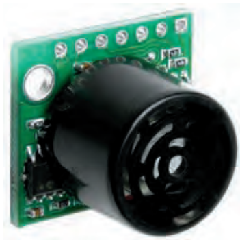
(c) Ultrasonic range finder Maxbotix LV-EZ3 (SparkFun SEN-08501)
