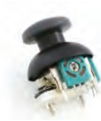
(b) Sparkfun joystick (COM-09032) and breakout board (BOB-09110)
