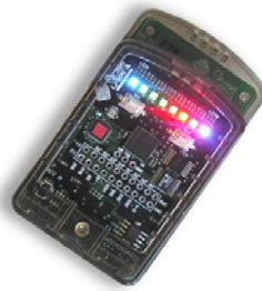
Sun SPOT (~2010): CPU: ARM ARM920T @ 180 MHz Flash: 512 KB RAM + 4 MB Flash Radio: 2.4 MHz IEEE 802.15.4
