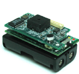
Mica Mote (~2004): CPU: Atmel ATmega 128 @ 4 MHz Flash: 128 KB RAM + 512 KB Flash Radio: 868/916 MHz
