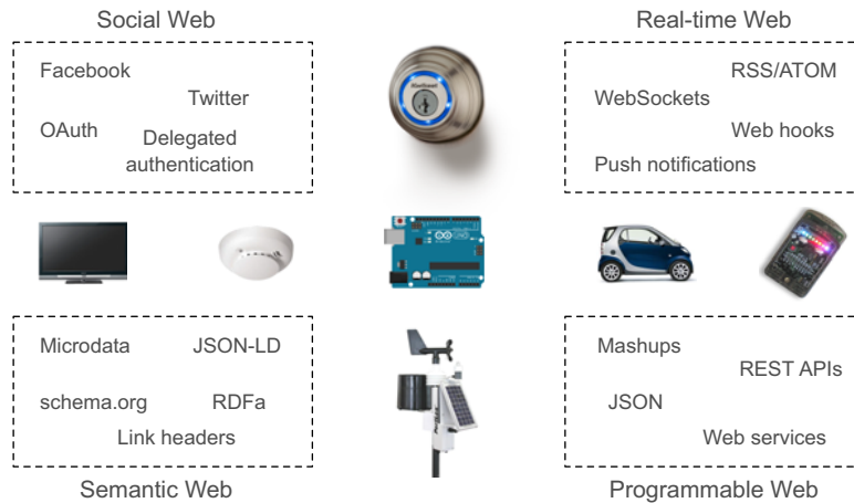
Figure 1.5 The Web of Things is the ability to use modern web standards on embedded devices. By using all these standards for Internet of Things scenarios, we both enable new types of interactive applications to be built and make sure that devices can be integrated with modern web applications and services with minimal effort.
