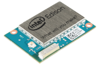
Intel Edison (~2014): CPU: Atom dual core @ 500 MHz Flash: 1 GB RAM + 4 GB Flash Radio: Wi-Fi + Bluetooth
