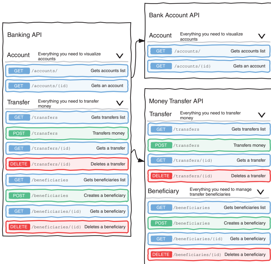
Figure 7.16 From one Banking API to separate Bank Account and Money Transfer APIs
