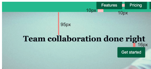
Figure 12.19 The design calls for 95 px above the slogan and 16 px beneath it (between it and the button).
