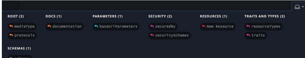
Figure 7.4 The Anypoint RAML editor features a bottom toolbar for adding sections to the schema model. This toolbar is context-sensitive; it will only offer appropriate sections based on where you are currently in the schema.
