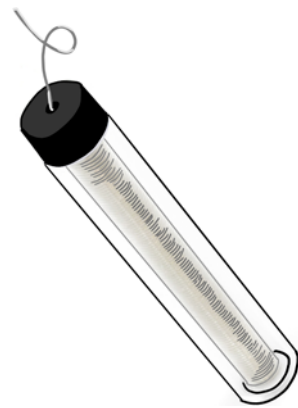
Figure 7.10 Solder comes on a wound spool, like thread.
