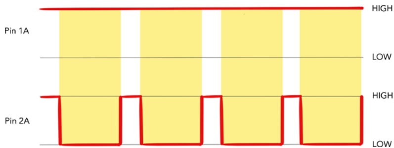
Figure 6.36 With direction set to HIGH (forward) on pin 1A and a 25% duty cycle on pin 2A (speed), the motor will be powered 75% of the time in the forward direction.
