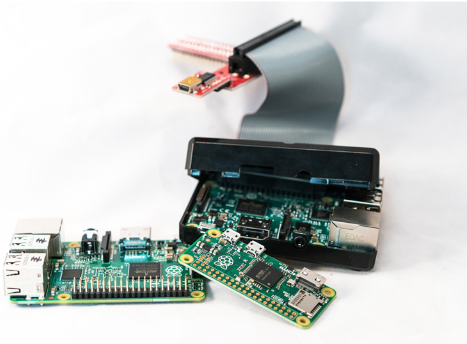
Figure 11.2 Raspberry Pi 2 Model B (left), Raspberry Pi Zero (center foreground), and Raspberry Pi 3 Model B (in a case, with attached SparkFun Pi Wedge)
