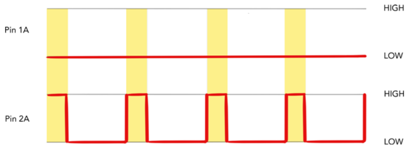
Figure 6.35 With direction set to LOW (reverse) on pin 1A and a 25% duty cycle on pin 2A (speed), the motor will be powered 25% of the time in the reverse direction.
