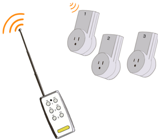
Figure 9.1 Sets of remote-controlled outlets are inexpensive and widely available at hardware stores and home centers. The remote control unit is powered by a low-voltage battery.
