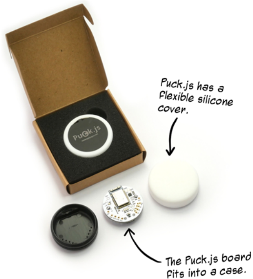
Figure 12.13 Puck.js is a BLE beacon device that—like the Pico—runs the Espruino JavaScript interpreter.
