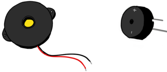
Figure 5.23 Some piezos have wire leads, and others have legs. Piezos have two pins: + and -.
