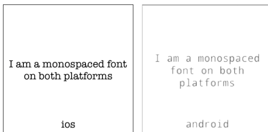
Figure 4.16 An example of rendering monospaced fonts on both iOS and Android
