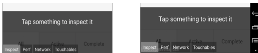
Figure 3.10 Using the inspector (left: iOS, right: Android)
