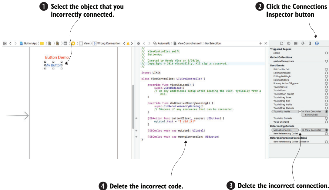
Figure 5.11 If you accidentally connected the objects to the code incorrectly, you need to delete the connection (wire) and the code following these steps.
