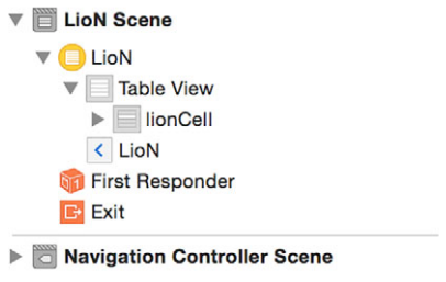
Figure 18.5 The Document Outline panel shows all the objects that are part of your storyboard.
