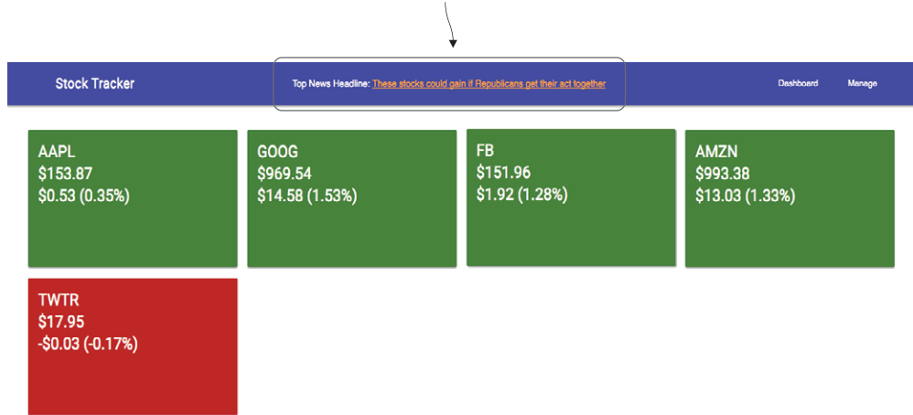
Figure 8.9 Example of an impure pipe that loads news at the top of the page by maintaining state in the pipe itself
